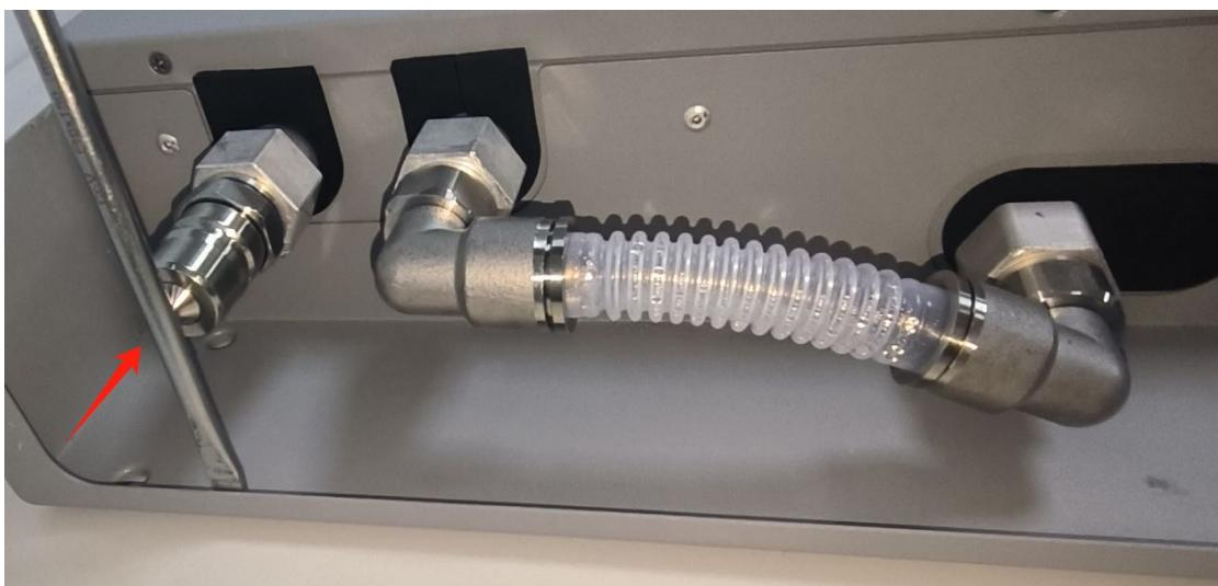
(4) Remove the corrugated hose as seen in the figure below. Press the movable ring of the quick-connect connector inwards, and then pull the corrugated hose out.
