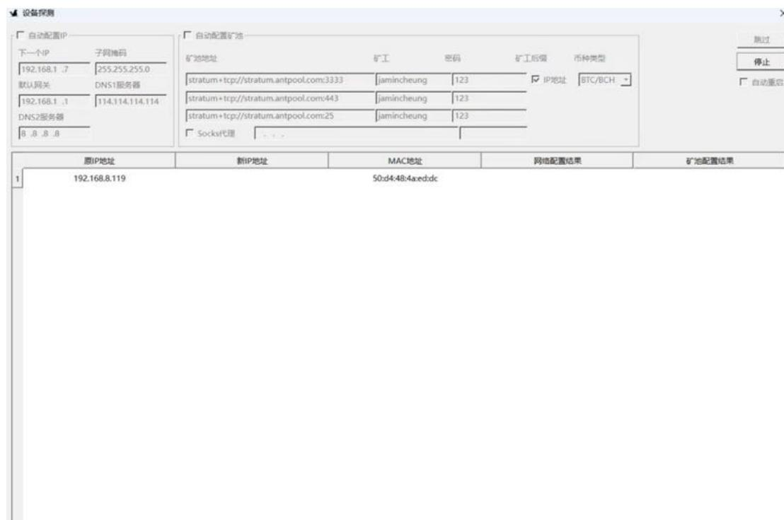
**Reporting IP method:** After starting the mining machine, press and hold the IP Report button on the mining machine for 5 seconds as seen in the figure below. Wait for a few seconds or until the current device IP is displayed on the software (Note: the management tool PC and the mining machine must be in the same LAN).
