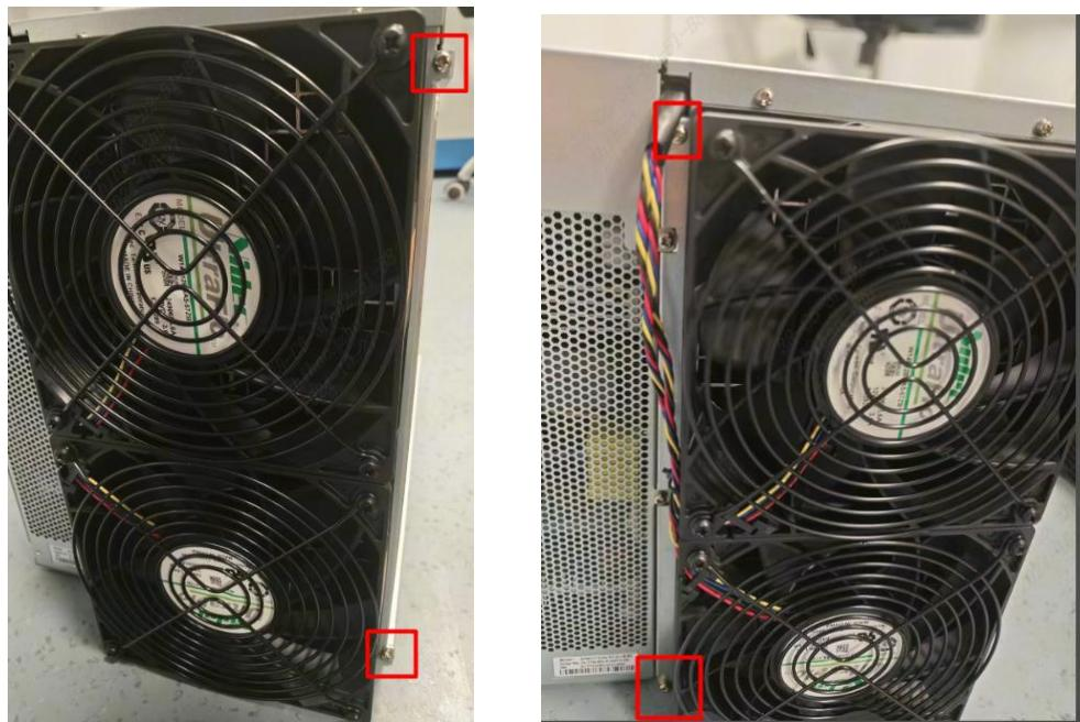
3. Pull out the cable of the hash board, unscrew two screws on the copper bar, and the hash board can be pulled out, as shown in the figure:
