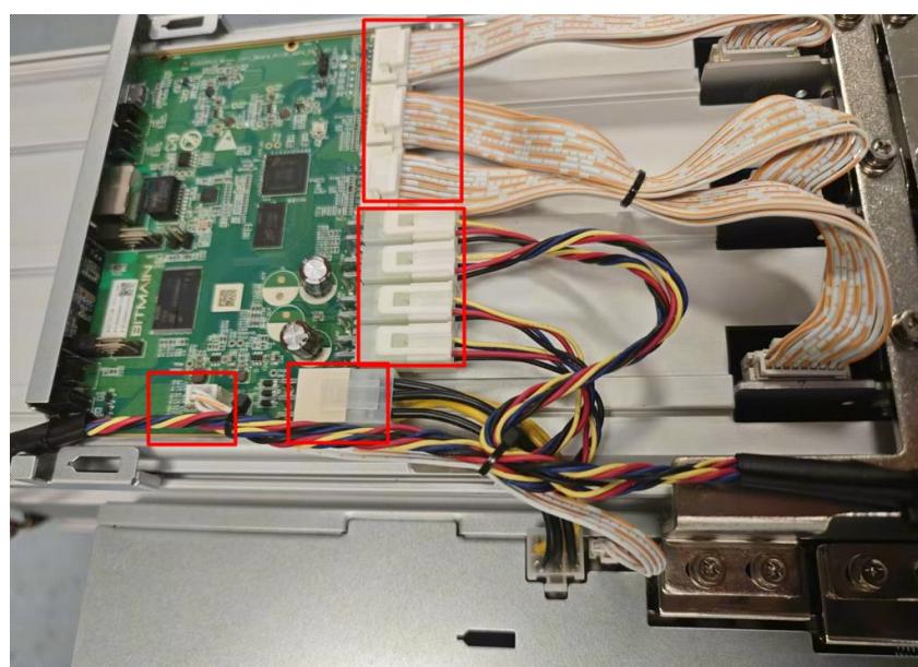
3. Remove 2 screws from the front cover of the control panel, remove the front cover, and push the control panel along the chute, as shown in the figure:
