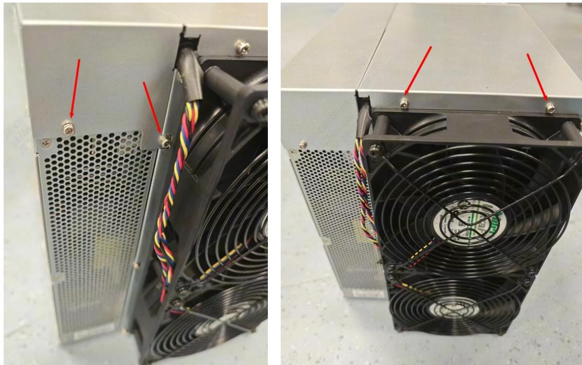
2. Remove the two upper covers and unplug a total of 9 cables on the control board, including the operation board arrangement cables, the fan cables, the control board power supply cables and the power supply voltage regulating cables, as shown in the figure:
