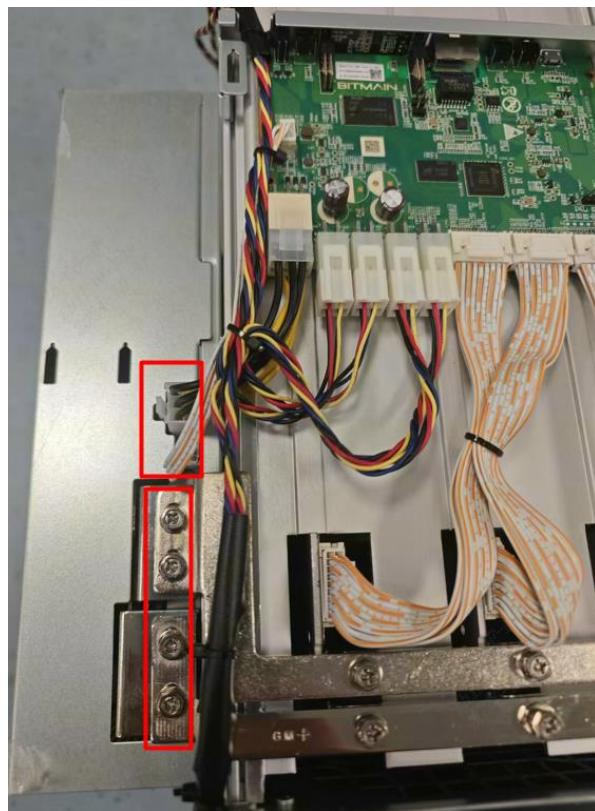
3. Remove the power supply and chassis fixing screws, as shown in the figure:
